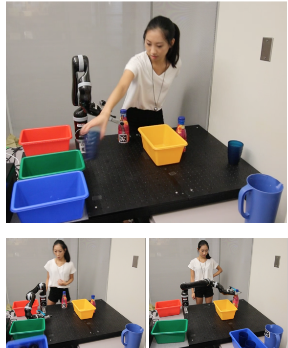
Figure 1: Top: User performs a repeated table-clearing task with the robot. The robot fails intentionally in the beginning of the task, in order to reveal its capabilities to the human teammate. Bottom-left: The robot drops the blue bin off the table while moving towards the left bottle. Bottom-right: The torques applied exceed their limits when the robot attempts a grasp at an extended configuration, and the robot stops moving.
