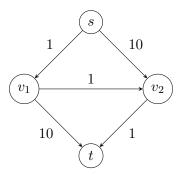
We seek to find the lowest-cost path from s to t. Because this search problem is represented by a directed acyclic graph, we will implement UCS as a tree search algorithm. The frontier will contain node, cost tuples, where the cost is the total cost from the start to the relevant node, and where nodes with lower cumulative cost have higher priority. Then UCS would thus proceed as follows:
