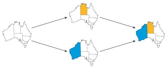
Backtracking search assigns the variables one by one, and backtracks if needed
