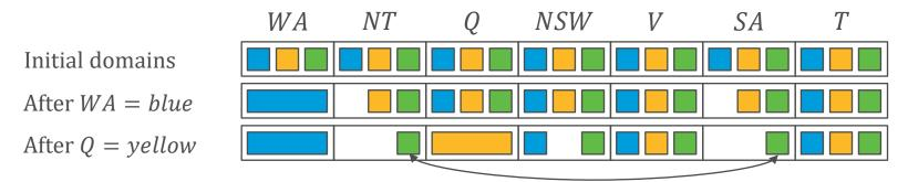
• The Inference function can implement AC-3, but only arcs  $(X_j, X_i)$  between the newly assigned variable  $X_i$  and unassigned neighbors  $X_j$  are initially added to the queue
