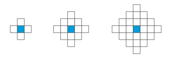
In a rectangular grid, search tree of depth d has  $4^d$  leaves, but there are only 4d states within d steps of any given state
