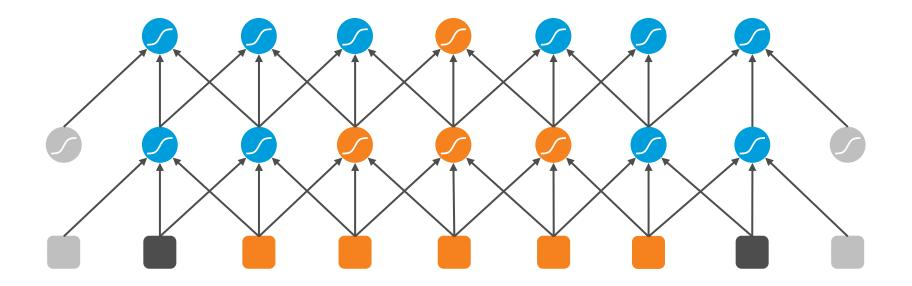
The receptive field of a unit is the portion of the input that can affect the unit. It is  $\ell$  in the first hidden layer but can be larger in deeper layers.
