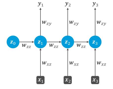
Diagram of a basic RNN where the hidden layer has recurrent connections
