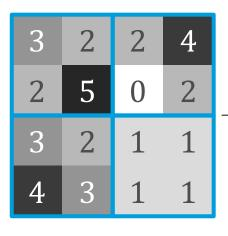
Average pooling with  $2 \times 2$  filters and s = 2
