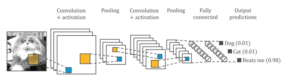
Different kernels correspond to different channels, and pooling is applied to each channel separately
