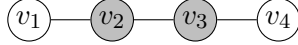
Figure 5: Graph illustrating that Mix-and-Match cannot provide an approximation ratio smaller than two. V_1 is shown in white, V_2 is shown in gray. Mix-and-Match returns the matching (v_2, v_3) .
