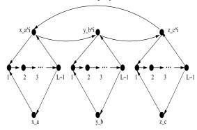
Figure 2: NP-completeness gadget for triple  $t_i$  and maximum cycle length L.
